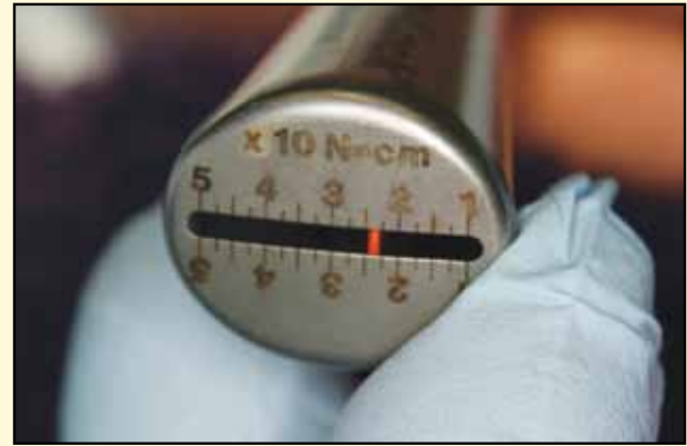
Figure 13: The implant torqued to over 50 Ncm, indicating excellent primary stability
